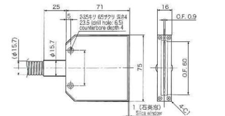
均一照射レンズ付き特殊ファイバ Special optical fiber with uniform radiation lens
